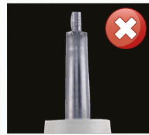
Worn screw thread with non genuine tips
