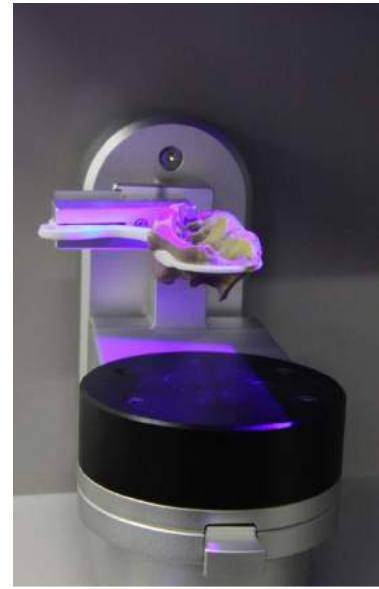
Put the impression on the impression jig and mount onto the scanner. Click [Auto scan] to proceed with scanning.
